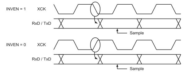
Using the inverted I/O (INVEN) setting for the corresponding XCK port pin, the XCK clock edges used for data sampling and data change can be selected. If inverted I/O is disabled (INVEN=0), data will be changed at the rising XCK clock edge and sampled at the falling XCK clock edge. If inverted I/O is enabled (INVEN=1), data will be changed at the falling XCK clock edge. For more details, see "I/O Ports" on page 139.
