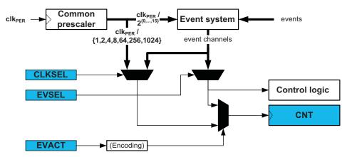
The peripheral clock is fed into a common prescaler (common for all timer/counters in a device). Prescaler outputs from 1 to 1/1024 are directly available for selection by the timer/counter. In addition, the whole range of prescaling from 1 to 2<sup>15</sup> times are available through the event system.
