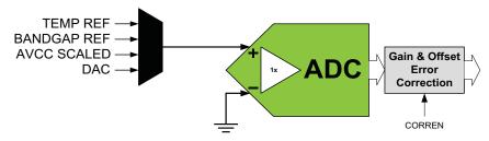
To measure the internal signals in unsigned mode, the negative input is connected to a fixed value given by the formula below, which is half of the voltage reference ( $V_{REF}$ ) minus a fixed offset, as it is for single-ended unsigned input. Refer to Table 25-2 on page 355 for details.
