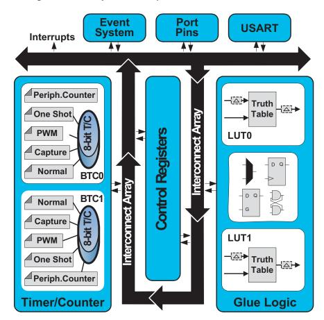
The timer/counter configuration allows for two 8-bits timer/counter usage. Each timer/counter supports normal, input capture, continuous and one shot pulse width modulations (PWM), with common flexible clock selections and event channels. By cascading the two 8-bit timer/counters, the XMEGA custom logic (XCL) offers a 16-bit timer/counter.
