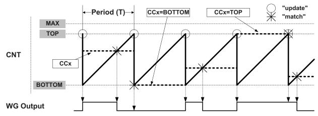
Figure 13-14.Single-slope Pulse Width Modulation
