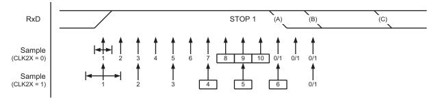
A new high-to-low transition indicating the start bit of a new frame can come right after the last of the bits used for majority voting. For normal speed mode, the first low level sample can be at the point marked (A) in Stop Bit Sampling and Next Start Bit Sampling. For double speed mode, the first low level must be delayed to point (B). Point (C) marks a stop bit of full length at nominal baud rate. The early start bit detection influences the operational range of the receiver.
