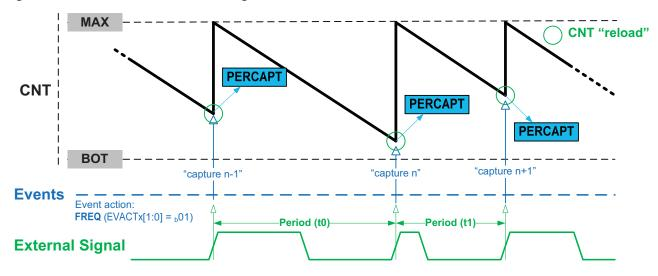
Figure 23-8. Timer/counter in CAPT Configuration with FREQ Command
