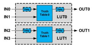
Figure 23-19.Two Independent 2-input LUT with Duplicated Input (2LUT1IN)
