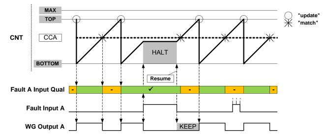
If the restart action is enabled, the timer/counter is halted as long as the fault condition is present and restarted when the fault condition is no longer present, as shown in Figure 16-12 on page 216. The compare channel output A is clamped to inactive level as long as the timer/counter is halted. Note that in RAMP2 mode of operation, when a new timer/counter cycle starts, the cycle index will change automatically.
