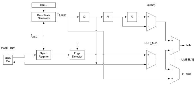
Figure 21-2. Clock Generation Logic Block Diagram
