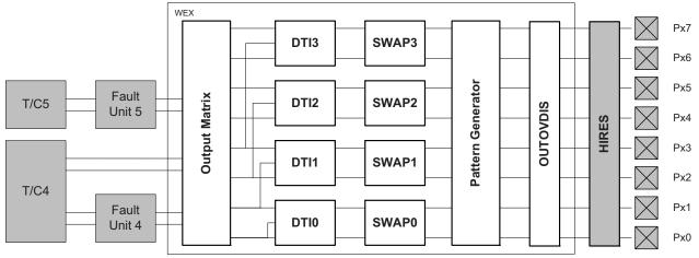
The output matrix (OTMX) can distribute and route out the waveform outputs from timer/counter 4 and 5 across the port pins in different configurations, each optimized for different application types.
