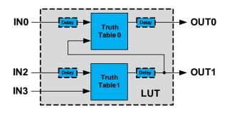
Figure 23-22.One 2-input Multiplexer Controlled by One 2-input LUT (MUX)
