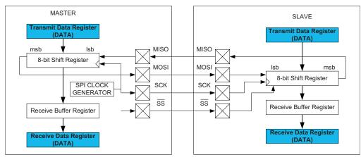
In SPI slave mode, the control logic will sample the incoming signal on the SCK pin. To ensure correct sampling of this clock signal, the minimum low and high periods must each be longer than two CPU clock cycles.
