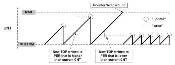
A counter wraparound can occur in any mode of operation when up-counting without buffering, as shown in Figure 13-8. This due to the fact that CNT and PER are continuously compared, and if a new TOP value that is lower than current CNT is written to PER, it will wrap before a compare match happen.
