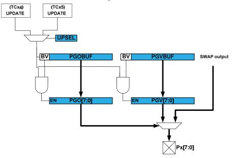
As with other double buffered timer/counter registers, the register update is synchronized to the UPDATE condition, set by the timer/counter waveform generation mode. If the synchronization provided is not required by the application, the application code can simply access the PGO, PGV, or PORTx registers directly.
