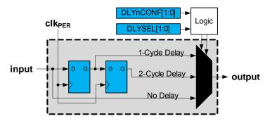
The insertion of a delay unit is selectable for each LUT, on the first of the two inputs or on the output. The insertion is decided by the application purpose, but some examples are provided:
