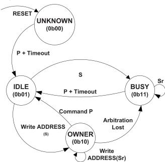
Figure 18-11.Bus State, State Diagram
