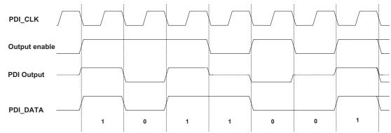
If the programmer and the PDI both drive the PDI\_DATA line at the same time, drive contention will occur, as illustrated in Figure 28-9. Every time a bit value is kept for two or more clock cycles, the PDI is able to verify that the correct bit value is driven on the PDI\_DATA line. If the programmer is driving the PDI\_DATA line to the opposite bit value to what the PDI expects, a collision is detected.
