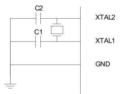
Two capacitors, C1 and C2, may be added to match the required load capacitance for the connected crystal.
