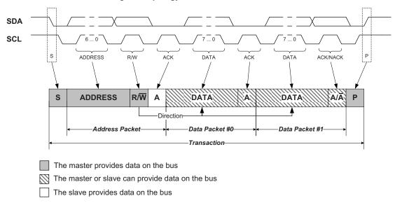
The master provides the clock signal for the transaction, but a device connected to the bus is allowed to stretch the lowlevel period of the clock to decrease the clock speed.
