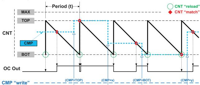
Figure 23-10.Single-slope Pulse Width Modulation
