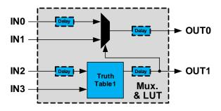
Figure 23-23.One D-Latch Controlled by Two 2-input LUT (DLATCH)
