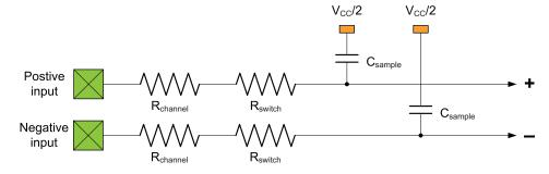
In order to achieve *n* bits of accuracy, the source output resistance, R<sub>source</sub>, must be less than the ADC input resistance on a pin:
