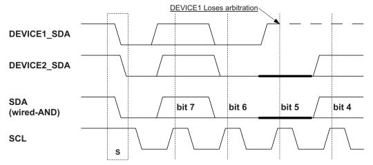
Figure 18-9 shows an example where two TWI masters are contending for bus ownership. Both devices are able to issue a START condition, but DEVICE1 loses arbitration when attempting to transmit a high level (bit 5) while DEVICE2 is transmitting a low level.
