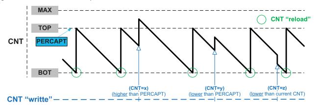
Figure 23-4. Counter in Normal Operation
