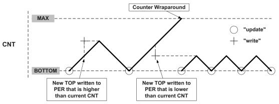
When double buffering is used, the buffer can be written at any time and still maintain correct operation. The period register is always updated on the UPDATE condition, as shown for dual-slope operation in Figure 13-9. This prevents wraparound and the generation of odd waveforms.
