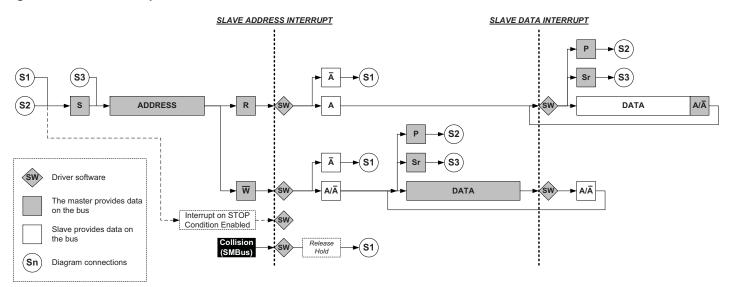
The number of interrupts generated is kept to a minimum by automatic handling of most conditions. Quick command can be enabled to auto-trigger operations and reduce software complexity.
