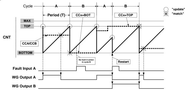
Figure 16-7. Waveform Generation with Restart Action in RAMP2 Mode
