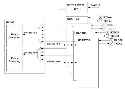
The IRCOM is automatically enabled when a USART is set in IRCOM mode. The signals between the USART and the RX/TX pins are then routed through the module as shown in Figure 22-1. The data on the TX/RX pins are the inverted value of the transmitted/received infrared pulse. It is also possible to select an event channel from the event system as input for the IRCOM receiver. This will disable the RX input from the USART pin.
