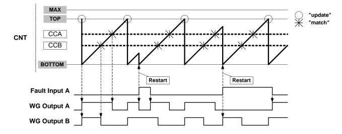
Note that in RAMP2 mode of operation, when a new timer/counter cycle starts, the cycle index will change automatically, as shown in Figure 16-7 on page 214. Fault A and fault B are qualified only during the cycle A and cycle B respectively, i.e. the compare channel outputs are not forced to inactive level as long as the fault condition is present in cycle B or cycle A respectively.
