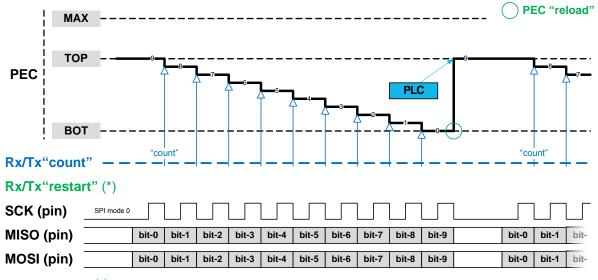
(\*) No Rx/Tx"restart": During PEC initialization for SPI communication, set-up PEC=PLC.
