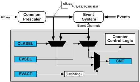
The peripheral clock is fed into the common pre-scaler (common for all timer/counters in a device). A selection of the prescaler outputs is directly available for both timer/counters. In addition the whole range from 1 to 2<sup>15</sup> times pre-scaling is available through the event system.
