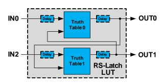
Figure 23-25.One DFF with Data Controlled by Two Independent 2-input LUT (DFF)
