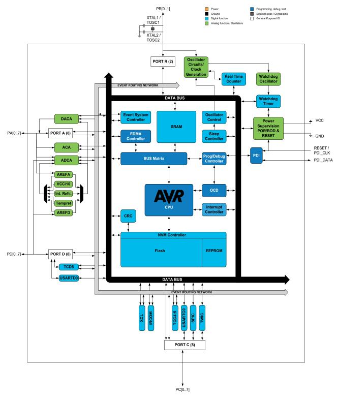
Note: 1. AV<sub>CC</sub> is only powering the following I/Os and analog functions: PA0 to PA7, AREF, ADC, DAC, AC0:1, Power Supervision, tempref, V<sub>REF</sub>, and Watchdog Oscillator. V<sub>CC</sub> is powering all other functions and I/Os.
