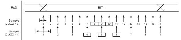
As for start bit detection, an identical majority voting technique is used on the three center samples for deciding of the logic level of the received bit. The process is repeated for each bit until a complete frame is received. It includes the first stop bit, but excludes additional ones. If the sampled stop bit is a 0 value, the frame error (FERR) flag will be set. Figure 21-8 shows the sampling of the stop bit in relation to the earliest possible beginning of the next frame's start bit.
