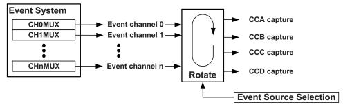
The event action setting in the timer/counter will determine the type of capture that is done.
