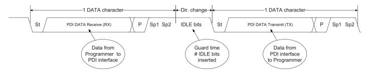
The external programmer will loose control of the PDI\_DATA line at the point where the PDI changes from RX to TX mode. The guard time relaxes this critical phase of the communication. When the programmer changes from RX mode to TX mode, a single IDLE bit, at minimum, should be inserted before the start bit is transmitted.
