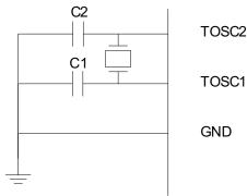
Two capacitors, C1 and C2, may be added to match the required load capacitance for the connected crystal. For details on recommended TOSC characteristics and capacitor load, refer to device datasheet.
