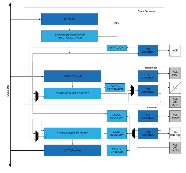
The clock generator includes a fractional baud rate generator that is able to generate a wide range of USART baud rates from any system clock frequencies. This removes the need to use an external crystal oscillator with a specific frequency to achieve a required baud rate. It also supports external clock input in synchronous slave operation.
