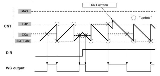
As shown in Figure 13-6, it is possible to change the counter value when the counter is running. The write access has higher priority than count, clear, or reload, and will be immediate. The direction of the counter can also be changed during normal operation.
