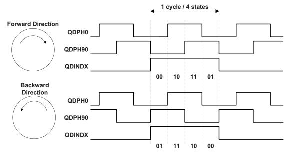
Figure 6-5 on page 86 shows typical quadrature signals from a rotary encoder. The signals QDPH0 and QDPH90 are the two quadrature signals. When QDPH90 leads QDPH0, the rotation is defined as positive or forward. When QDPH0 leads QDPH90, the rotation is defined as negative or reverse. The concatenation of the two phase signals is called the quadrature state or the phase state.
