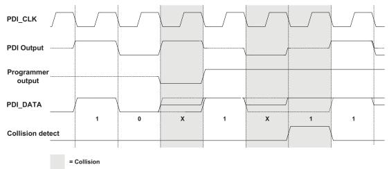
As long as the PDI transmits alternating ones and zeros, collisions cannot be detected, because the PDI output driver will be active all the time, preventing polling of the PDI\_DATA line. However, the two stop bits should always be transmitted as ones within a single frame, enabling collision detection at least once per frame.
