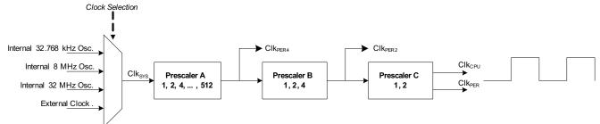
Prescaler A divides the system clock, and the resulting clock is  $clk_{PER4}$ . Prescalers B and C can be enabled to divide the clock speed further to enable peripheral modules to run at twice or four times the CPU clock frequency. If Prescalers B and C are not used, all the clocks will run at the same frequency as the output from Prescaler A.
