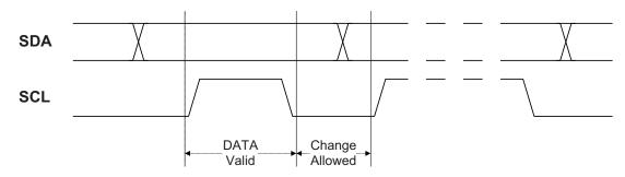
Combining bit transfers results in the formation of address and data packets. These packets consist of eight data bits (one byte) with the most-significant bit transferred first, plus a single-bit not-acknowledge (NACK) or acknowledge (ACK) response. The addressed device signals ACK by pulling the SCL line low during the ninth clock cycle, and signals NACK by leaving the line SCL high.
