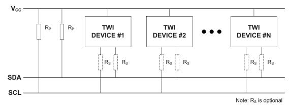
An unique address is assigned to all slave devices connected to the bus, and the master will use this to address a slave and initiate a data transaction.
