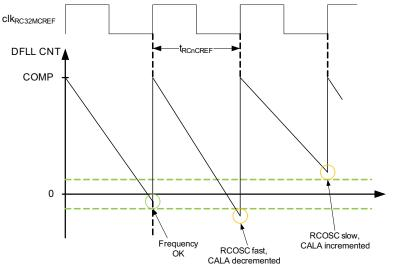
The DFLL will stop when entering a sleep mode where the oscillators are stopped. After wake up, the DFLL will continue with the calibration value found before entering sleep. The reset value of the DFLL calibration register can be read from the production signature row.
