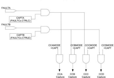
CAPTURE LOGIC in FMODE2 FAULT Mode (TCx.CTRLD.EVACT[2:0] = 010)
