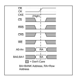
A subsequent ACTIVE command to another bank can be issued while the first bank is being accessed, which results in a reduction of total row-access overhead. The minimum time interval between two successive ACTIVE commands on different banks is defined by trrd.
