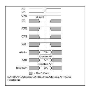
The basic Read timing parameters for DQs are shown in following figure; they apply to all Read operations.
