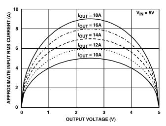
FIGURE 10. SWITCHING CONVERTER RMS INPUT CURRENT
