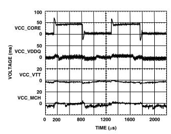
FIGURE 9. HIP6020EVAL1 OUTPUT TRANSIENT RESPONSE
