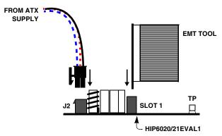
FIGURE 2. QUICK START EVALUATION CONNECTIONS
