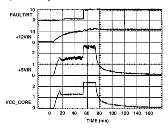
FIGURE 5. START-UP SEQUENCE WITH SHORTED Q1 (ATX CONTROL CIRCUIT BY-PASSED)
