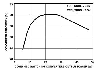
FIGURE 8. HIP6021EVAL1 MEASURED CONVERTER EFFICIENCY
