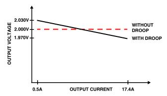
FIGURE 4. OUTPUT VOLTAGE DROOP AT 2.0V DAC SETTING
