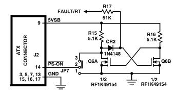
FIGURE 3. ATX POWER SUPPLY CONTROL CIRCUIT
