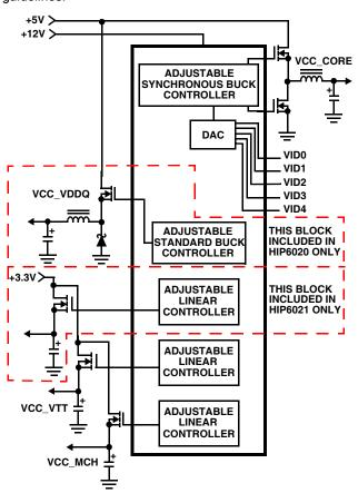
FIGURE 1. HIP6020/21EVAL1 BLOCK DIAGRAM
