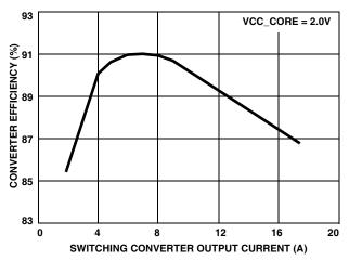
FIGURE 7. HIP6021EVAL1 MEASURED CONVERTER EFFICIENCY
