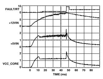
FIGURE 6. START-UP SEQUENCE WITH SHORTED Q1 (ATX CONTROL CIRCUIT ACTIVE)
