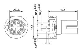
M12 female connector contact carrier
