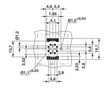
Soldering pad geometry
