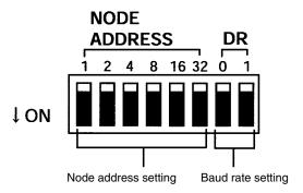
Note Set the same baud rate on all nodes (Master and Slaves) in the network. If the F150 is not set to the correct baud rate, it will be unable to participate in the network and communications errors may occur in communications between nodes with correct node address settings.
