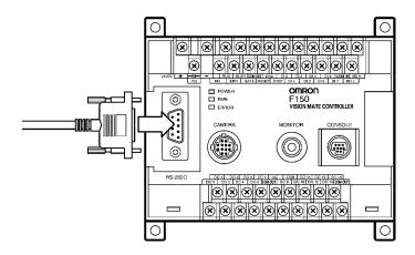
**Note** Always tighten the connector screws.
