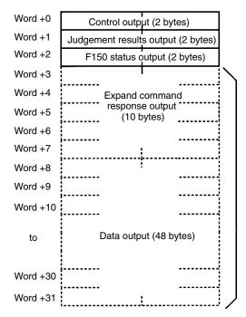
These outputs can be enabled or disabled. When the "expand command response output" is disabled, the data output will be shifted up to word +3.
