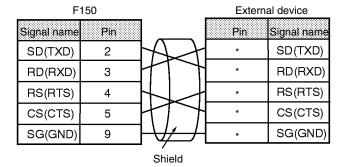
**Note** Pin numbers on the external device will depend on the device being connected. Refer to the manual for the device being connected.
