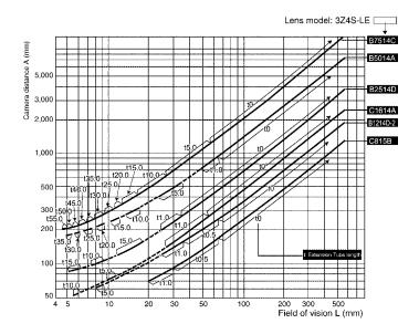
The X axis of the graph shows field of vision L (mm), and the Y axis shows the camera distance A (mm). The curves on the graph indicate different lenses, and the "t" values indicates the lengths of the Extension Tubes.
